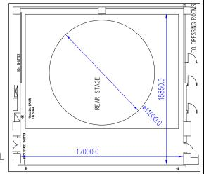
The rear stage fire shutter is treated as a safety curtain by FSD and cannot be obstructed by scenery, equipment or stage wagon in production.
