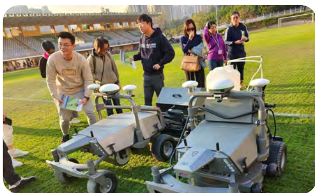
Demonstration of an autonomous robotic mower with line-marking function for trainees of a turf-grass training course.
